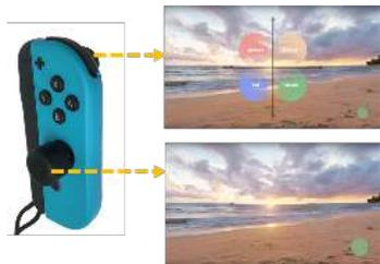
(b) Joy-con Right Controller (Joystick for rating emotion and Trigger Button for activating helper function).
