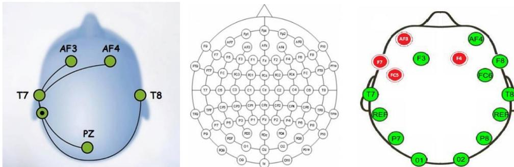
Figure 1: (a) Position of 5 sensors of the Emotiv Insight helmet (Emotive Pro manual); (b) Example of location of 74 sensors of Modified combinatorial nomenclature of the 10-10-system standard, but also a limitation in the information detected: “measurements taken with the Emotiv Insight do not prove to be reliable for a classification task as simple as right versus left motor activity and that the device is not recommended as a Brain Computer Interface” [22].
